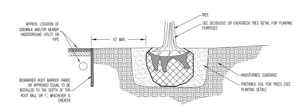
1. ANY TREE INSTALLED WITHIN 10 FT. OF NEW CONCRETE SIDEWALKS SHOULD BE INSTALLED WITH BIOBARRIER
