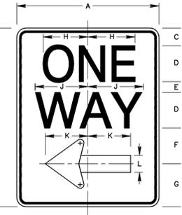
(A) JUSTIFICATION. THE VERTICAL ONE-WAY SIGNS (R6-2L) & (R6-2R) SHALL BE AUTHORIZED FOR USE ONLY WHEN LATERAL SPACE IS LIMITED, IN LIEU OF THE HORIZONTAL ONE-WAY SIGNS (R6-1L) & (R6-1R) AND FOR OVERHEAD INSTALLATIONS.
