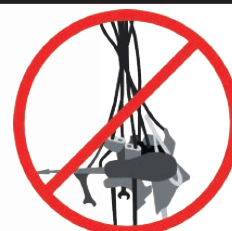
Tool assemblies are spaced to prevent tangling
