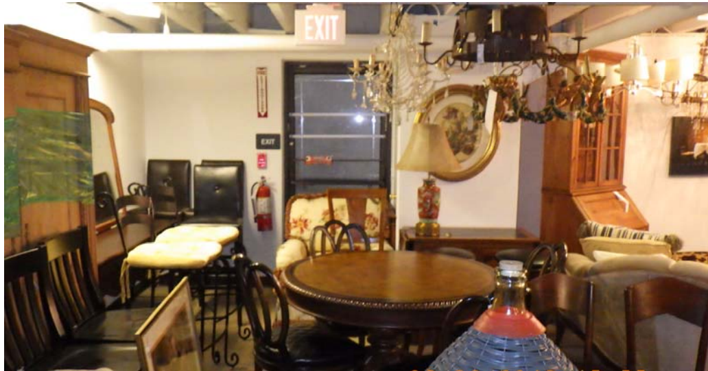
Emergency Exit Blocked
